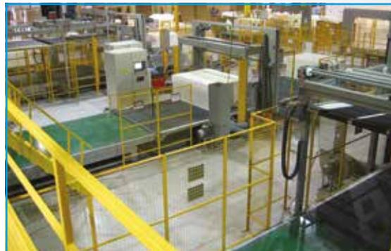
Three W 22 splitting and stacking machines in production.
