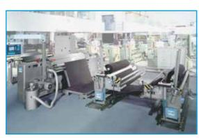
Splitting Machine G 11 with wind-up and wind-off device.
