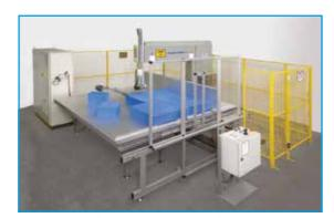
Vertical Bandknife Cutting Machine V 51/5.
