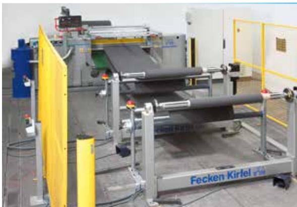
**K 21 with winder:** In order to use the K or D machines for roll goods, they can be equipped with conveyor belts and winding devices.
