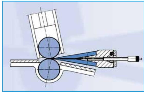
The following applies for all K and D types: The bandknife tip is automatically adjusted with the aid of a light barrier and a servomotor. The ratio between the material to be cut, the feed rollers, the knife tip, and the knife guide remains constant. This means that a consistent cut quality is achieved over the entire lifespan of the bandknife.
