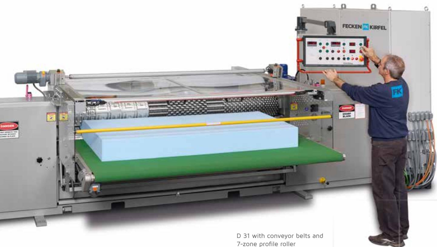
D 31 with conveyor belts and 7-zone profile roller
