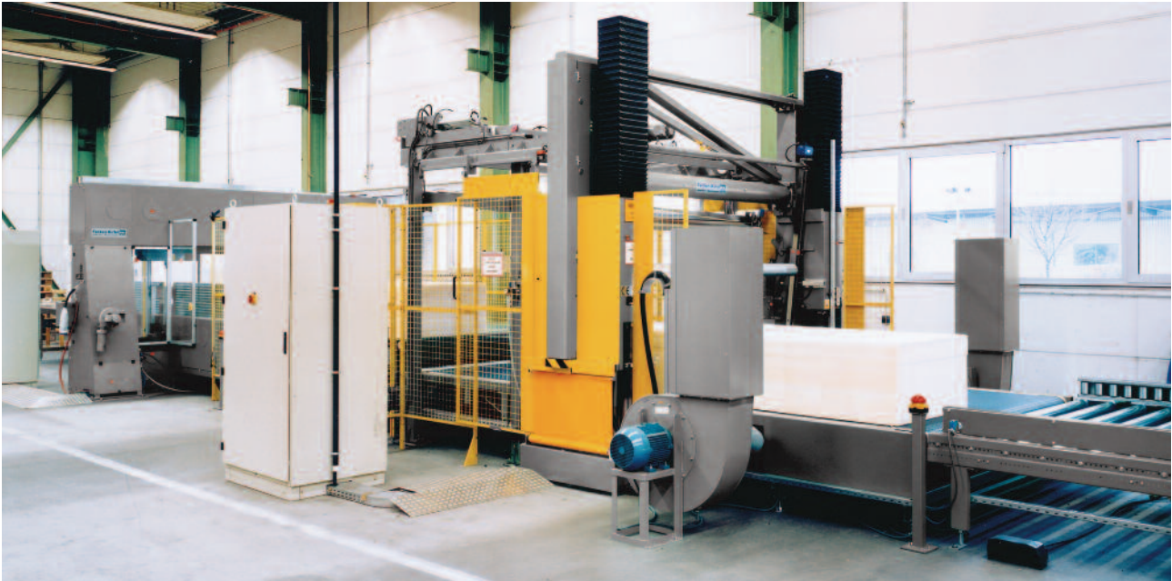
Automatic Horizontal Splitting and Stacking Machine H 52 with Vertical CNC Contour Cutting Center F 52
