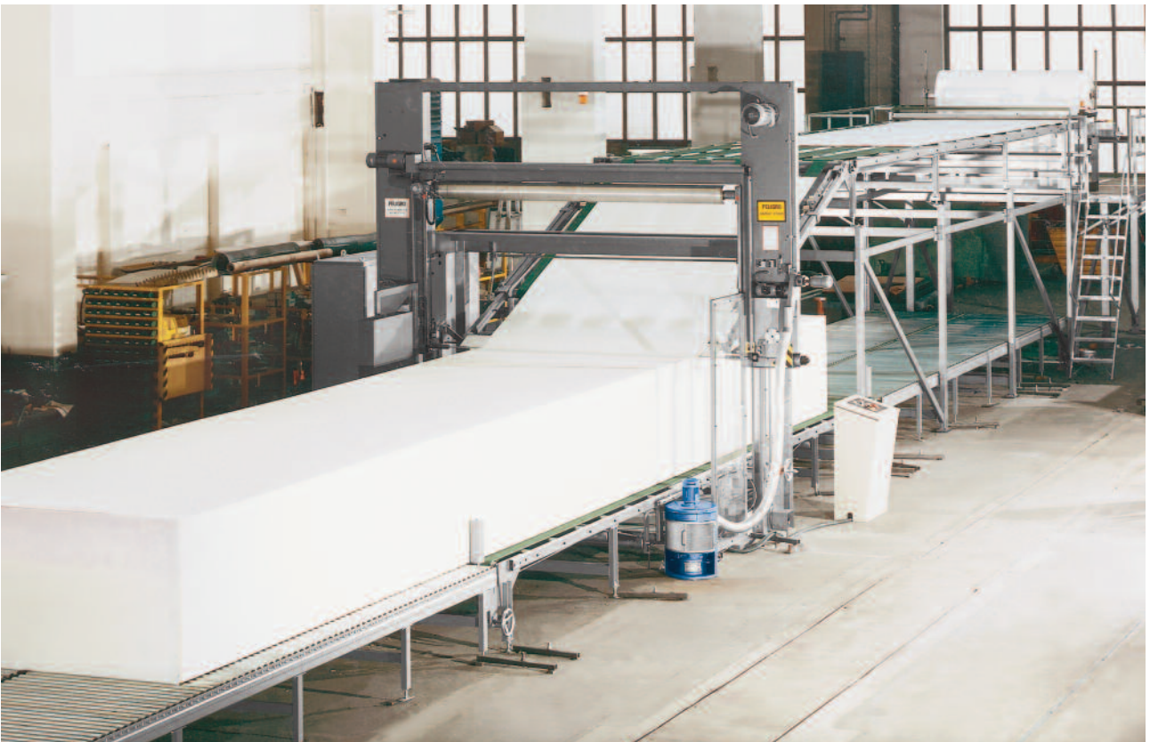
Machine W 22 with conveyor belt and wind-up machine A 4
