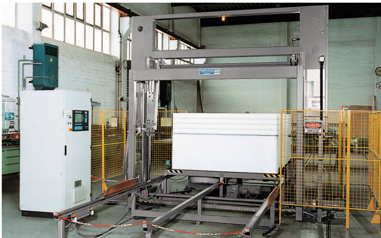
Automatic Horizontal Splitting and Stacking Machine W 21 with sliding table
